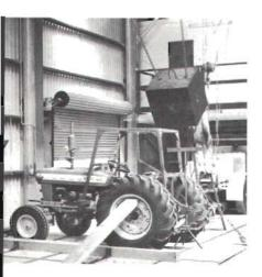
Impact testing of the protective frame on a tractor at the University of Melbourne's tractor testing station at Werribee.
